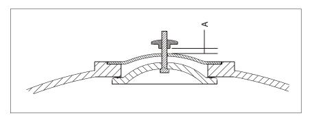
Once the filter has been completely filled with water, start the performance of installation, venting manually to eliminate all the air that could be inside the filter, as the presence of air impairs the filter performance.
