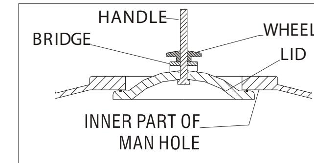
Introduce the lid in the man hole, leaving it leveled and centered. The lid must be supported by the handle, as this will avoid that it could fall into the tank and damage any of its parts.
