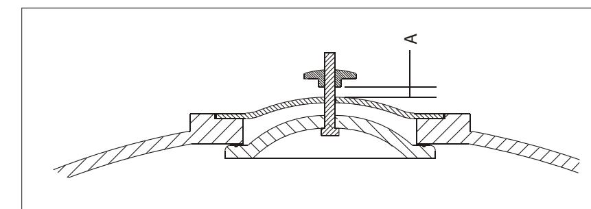
Once the filter has been completely filled with water, start the performance of installation, venting manually to eliminate all the air that could be inside the filter, as the presence of air impairs the filter performance.
